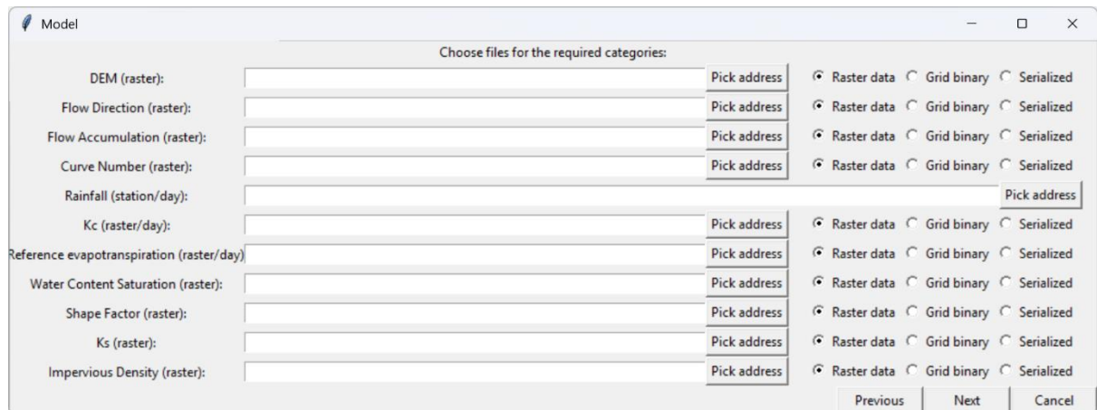
Figure 2. DT-Agro GUI, selection of input datasets for each required category (DEM, flow direction, rainfall, Kc, etc.) and choice of file format (raster, grid binary or serialized).
